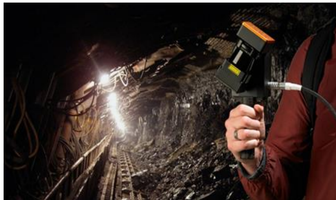
Figure 9. GeoSLAM Zeb-Revo handheld scanner (Image from GeoSLAM Brochure)
